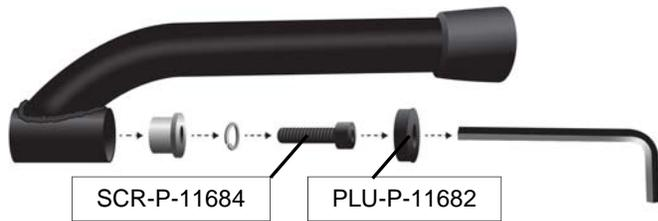
6mm Allen wrench is used for both assembly types. Keep wrench to remove or re-tighten legs as needed.
